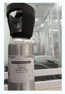
CRM No: IDNRM-MG-1-014 **Description :** CO<sub>2</sub> in N<sub>2</sub> Form/Size : 50 bar, 4 L/cylinder Analyze and Certified Value & **Uncertainty**: CO<sub>2</sub>: (2.78 ± 0.02) %mol/mol
