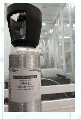
CRM No : IDNRM-MC-1-001 Description : CO<sub>2</sub> in N<sub>2</sub> Form/Size : 100 bar, 4 L/cylinder Analyze and Certified Value & **Uncertainty**:
