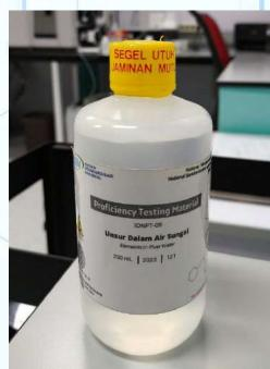
CRM No : IDNRM-MI-2-001 Description : Elements in river water Form/Size : Liquid 250 mL/bottle Analyze and Certified Value & Uncertainty : As :  $(24.0 \pm 1.3) \mu g/L$ Cd :  $(4.50 \pm 0.29) \mu g/L$ Fe :  $(239 \pm 15) \mu g/L$ Mn :  $(123.5 \pm 5.7) \mu g/L$ Zn :  $(73.9 \pm 4.5) \mu g/L$ Clasified CRM or RM) : CRM Institute service identifier : MI-1
