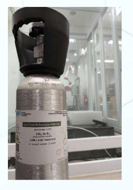
**CRM No**: IDNRM-MG-1(on demand) **Description :** CO<sub>2</sub> in N<sub>2</sub> **Form/Size :** 100 bar, 4 L/cylinder Analyze and Certified Value & **Uncertainty**: CO<sub>2</sub> : 1 - 500 mmol/mol (± 0.65% relative) CRM No: IDNRM-MG-1(on demand) **Description :** CO<sub>2</sub> in N<sub>2</sub> Form/Size : 100 bar, 4 L/cylinder Analyze and Certified Value & **Uncertainty**:
